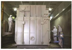
The surface treatment of raw materials in initial stage as well as semi-completed tanks are carried out by shot blasting process.
